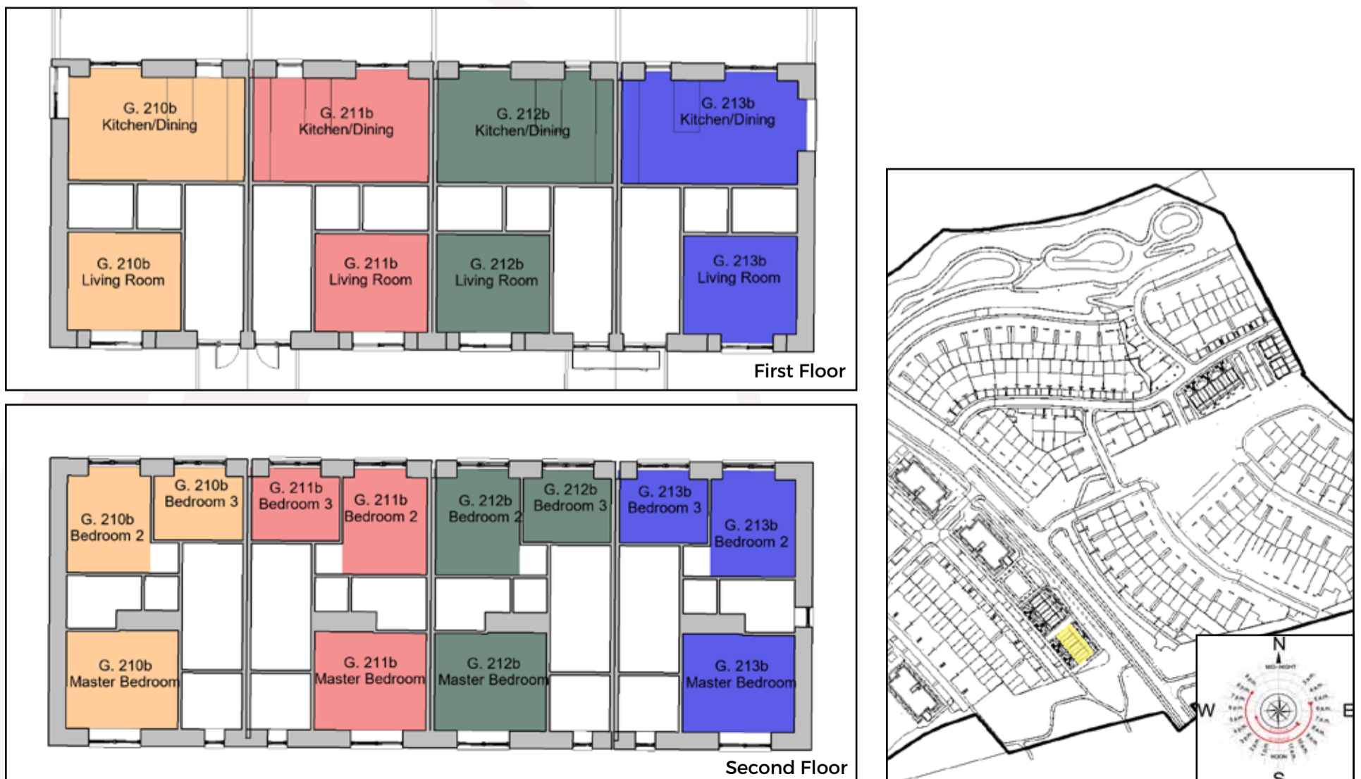
Figure H.19: Floor plans of assessed building (L), Keyplan highlighting the assessed building (R).
