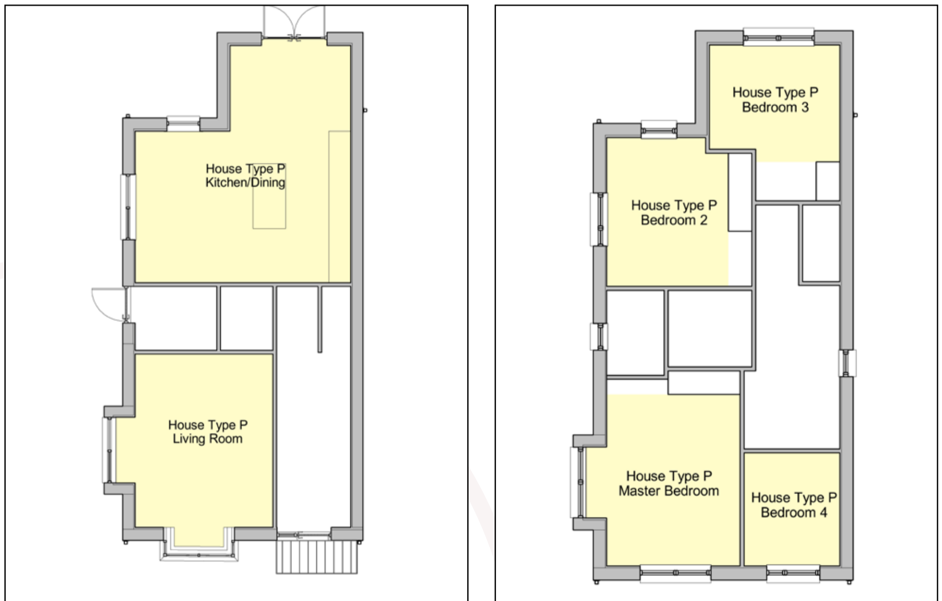
Figure I.4: Floor plans of the assessed house type. Ground Floor (L), 1st Floor (R).
